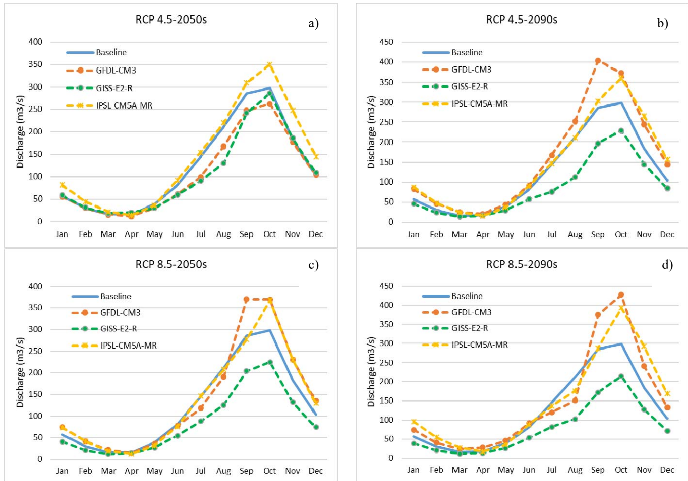
Figure 4.3: Monthly projected streamflow under 2RCPs from 3GCMs for 2050s and 2090s at outlet of basin (sub-basin 42)
